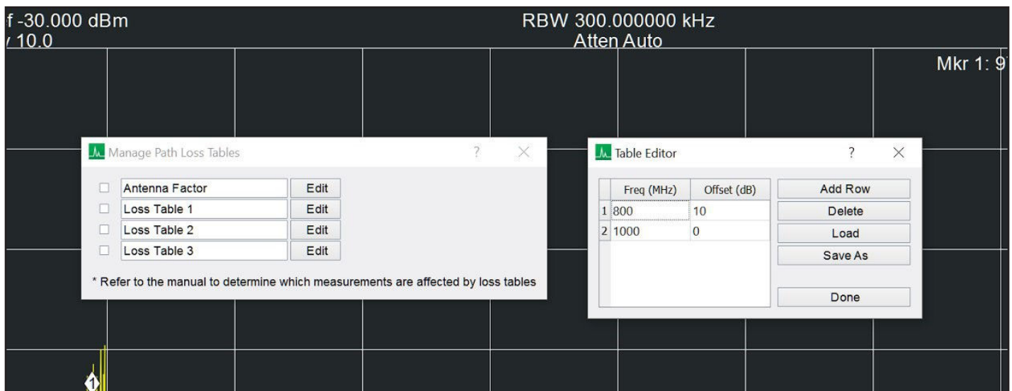
Figure 3—Up to 3 Path Loss Tables and 1 Antenna Factor Correction Table are accessible through the Path Loss Table Manager in Spike, where the tables can be manipulated by Add Row , Delete Row , Load , and Save As features.
