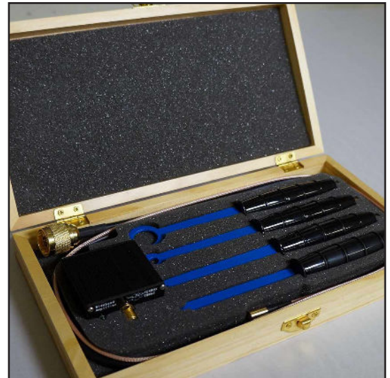
Figure 6—A set of near-field probes for performing radiated emissions EMC pre-compliance measurements.
