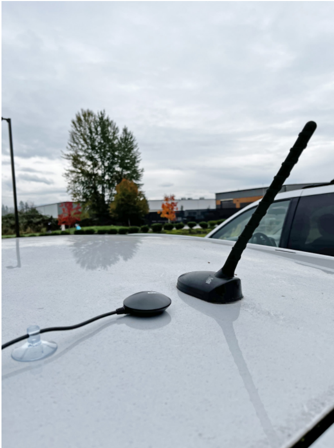
Figure 3: An external GPS unit on roof of vehicle, next to antenna.
