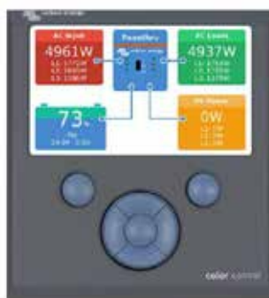
Color Control GX, showing a PV application
